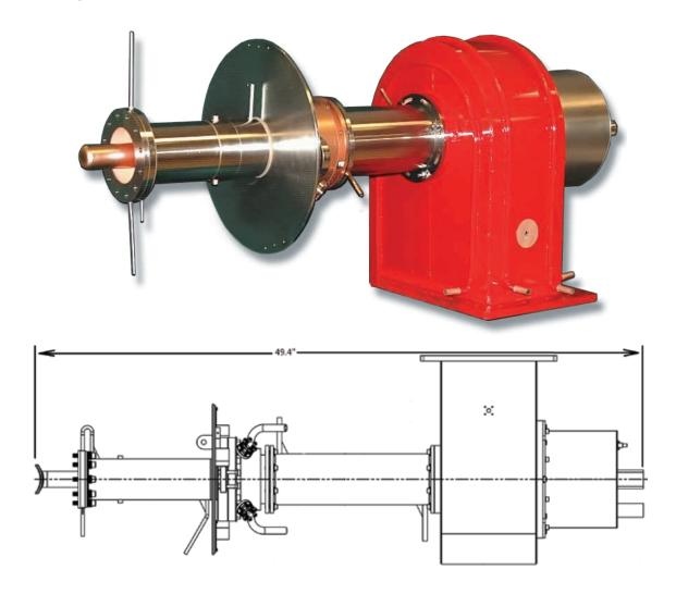
The VWP3070 Fundamental Power Coupler was designed for the Brookhaven FEL injector. All components of the coupler are water cooled to handle the high RF power. The design utilizes a TiN coating for multipactor suppression, and high RRR copper plating for low RF loss.
